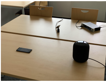
Figure 1: Examples of the experimental setup and recorded vibrations. Accelerometer measurements (blue) and sound (orange) were recorded while playing an 18Hz sine wave at 84dB and 64dB SPL in 50cm between devices. The figure shows the raw signal and its FFT representation. A clear peak at 18Hz is clearly distinguishable in the FFT values even for the low SPL.
